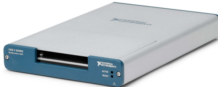
Figura 2.1: Scheda National Instruments USB-6341
